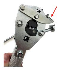
**3.** Push the tube up to the arm which indicates how far to push the tube through before flaring.
