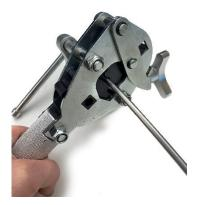
**4.** Clamp the tube down by rotating the handle until tight, ensuring the tube does not move.
