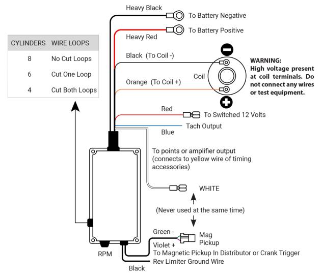
**WARNING:** During installation disconnect the battery cables. Always remove the negative cable first and install it last.
