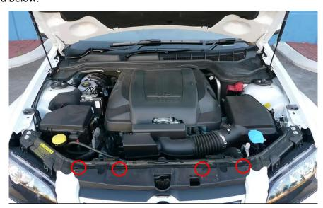
**3.** Remove the top radiator mounts by lifting the tab located in the centre of the mount. You can use a flat head screw driver by inserting into the mount and pulling the tab forward to release. Move mount side to side and lift vertical off the mounting rails.
