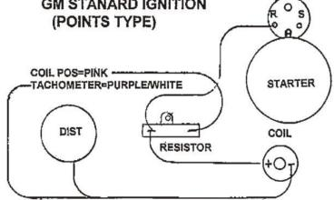
NOTE: POINTS TYPE IGNITION SYSTEMS REQUIRE A BALLAST RESISTOR TO LOWER VOLTAGE TO THE COIL AND EXTEND POINT LIFE. FORD & MOPAR USE A RESISTOR WIRE ORIGINALLY FOR THIS, BUT YOU CAN SUBSTITUTE WITH THE CERAMIC TYPE. IT IS IMPORTANT TO ALSO INSTALL A BY-PASS WIRE SO THAT THE COIL WILL HAVE FULL VOLTAGE WHEN THE ENGINE IS CRANKING. FOR GM USE THE
